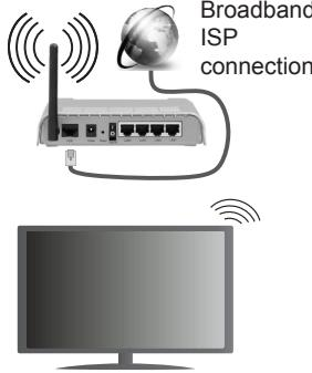
A Wireless-N router (IEEE 802.11a/b/g/n) with simultaneous 2.4 and 5 GHz bands is designed to increase bandwidth. These are optimized for smoother and faster HD video streaming, file transfers and wireless gaming.
